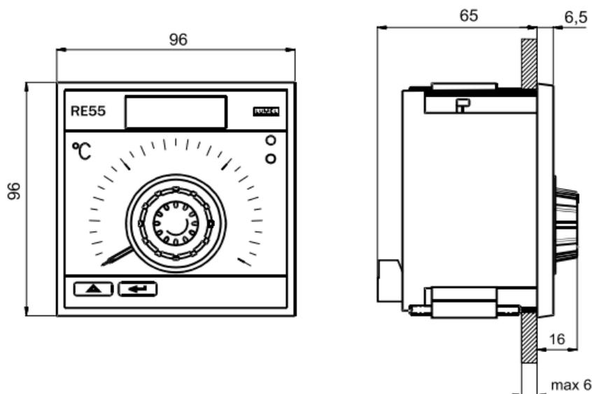
Fig.2. Overall dimensions of the RE55 controller.
