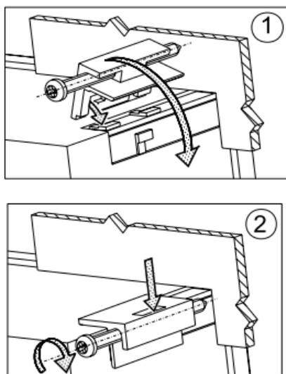
Fig. 1. Way of controller fixing.
