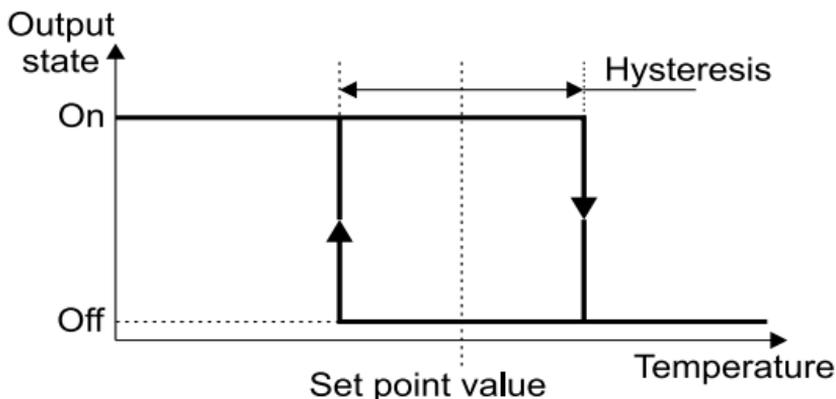
Fig.8. Operation way of the output heating type.
