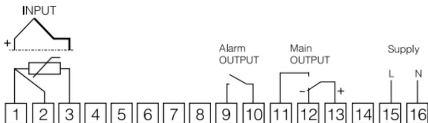
Fig. 3. Scheme of electrical connections.
